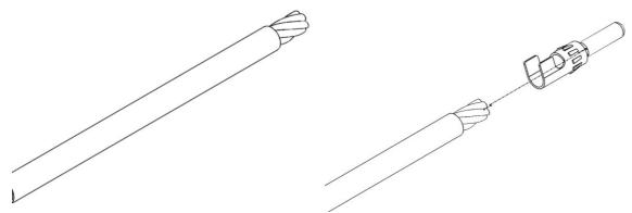
2. Insert base of MC4 connector through wire then tighten with head of MC4
