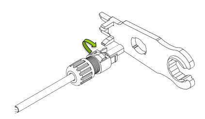
4. Use the second MC4 tool to grip the base of the MC4 connector. Rotate one of the tools while keeping the other still to finish tightening the MC4 connector
