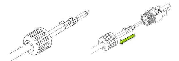
3. After initial tightening, insert the nose of the MC4 connector head through the middle hole of the MC4 tool
