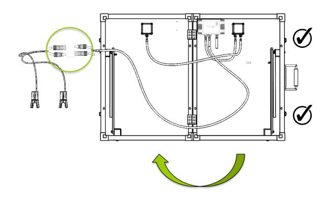
2. Connect Battery Alligator Clips to 12V Battery
