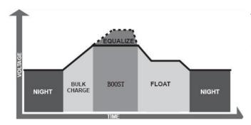
**Bulk Charge:** This algorithm is used for day to day charging. It uses 100% of available solar power to recharge the battery and is equivalent to constant current.
