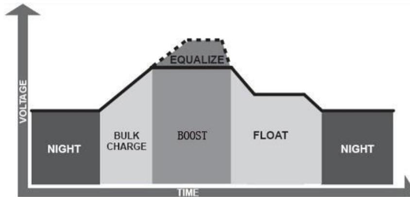
**Bulk Charge:** This algorithm is used for day to day charging. It uses 100% of available solar power to recharge the battery and is equivalent to constant current.
