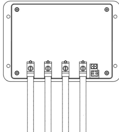
**3. Insert Temperature Sensor block terminal and connect wires
