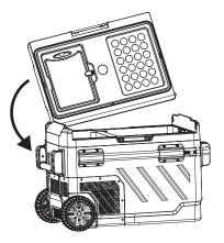
(5) Align the door shaft with the hole on one side and insert it.
