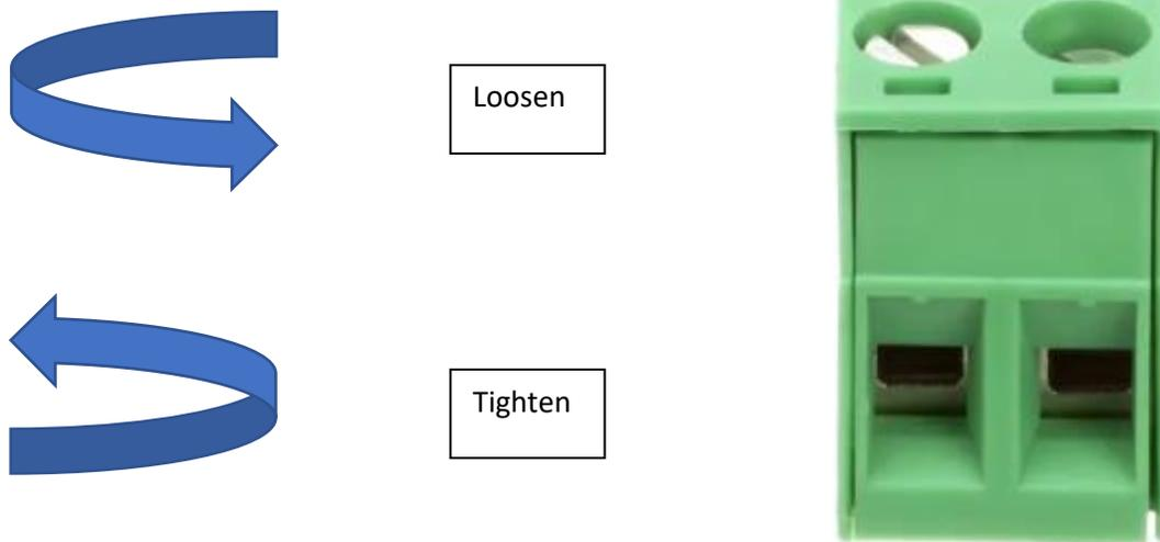
3. In this example we are connecting to the Left (positive, +) and Right (negative, -) convention if facing the terminal block like in the example above. Proceed to connect the positive pin from the RVSCC and rotate clockwise to clamp on the wire. Repeat for the negative connector.
