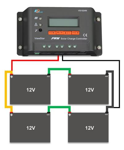
Figure 9.6 Four 12V batteries connected in series - parallel
