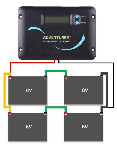
Figure 9.3 Four 6V batteries connected in series - parallel
