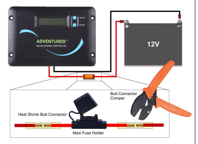
The butt connectors recommended for this application are the type with heat shrink insulation. This will keep will give extra protection for the internal connection.
