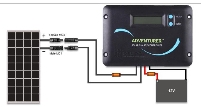
Figure 6.4 Completed 12V off-grid system
