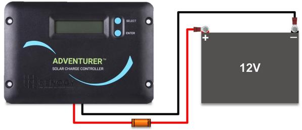
Figure 6.1 Charge controller connected to a 12V battery
