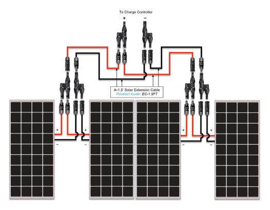
Figure 8.5 Four RNG-100D Panels in parallel
