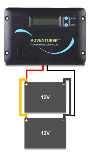
Figure 9.2 Two 12V batteries connected in parallel
