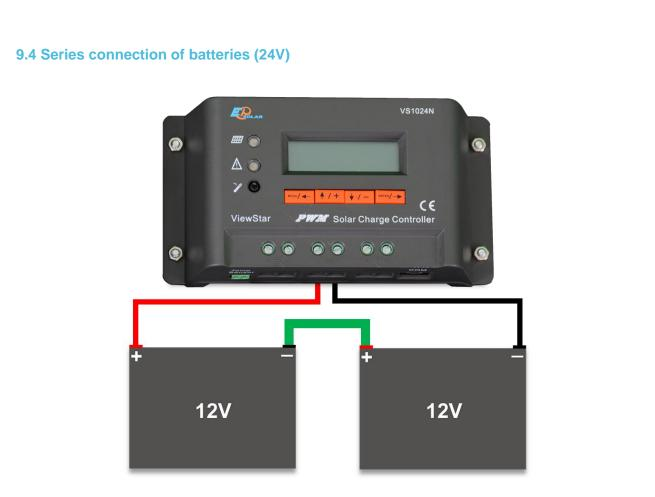
Figure 9.4 Two 12V batteries connected in series
