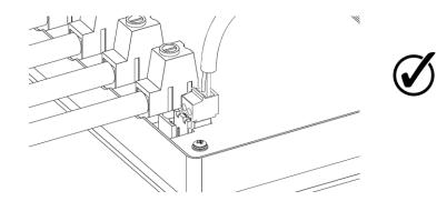
4. Insert battery remote sensor block terminal and connect wires (POLARITY SENSITIVE)
