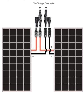
Figure 8.2 Two RNG-100D Panels in parallel
