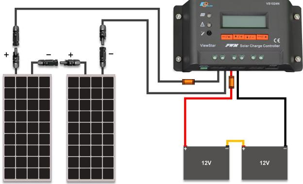
Figure 7.1 Completed 24V off-grid system
