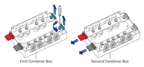
**Step 2:** Align the busbar ports.
