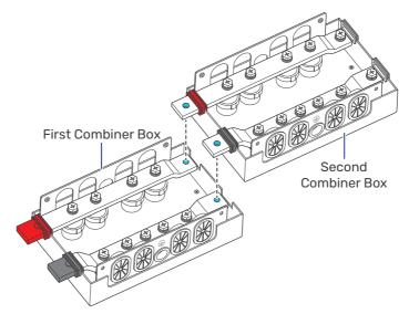
Step 3: Install the terminal bolts, spring washers, and flat washers on the busbar ports.
