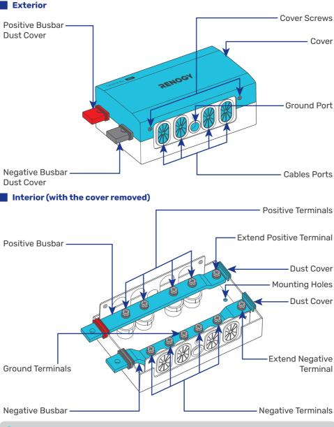
Each busbar terminal is equipped with a terminal bolt, a spring washer, and a flat washer.
