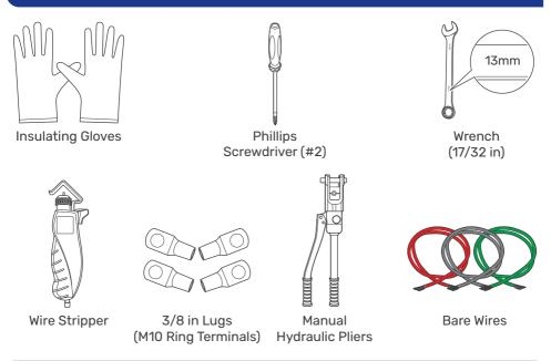
Prior to installing and configuring the combiner box, prepare the recommended tools, components, and accessories.
