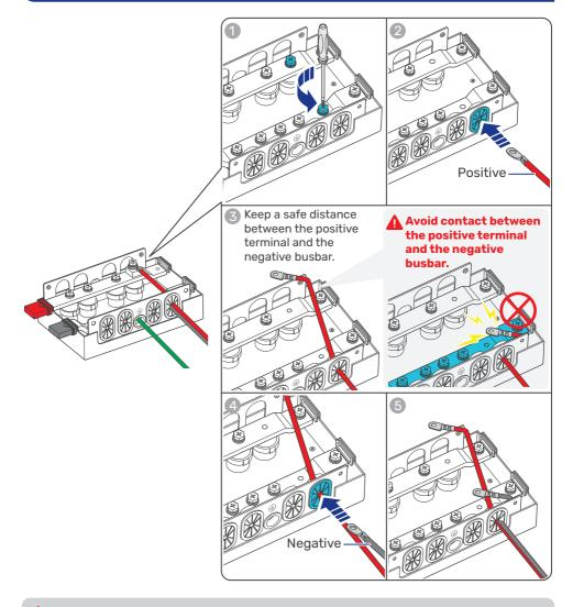
Ensure that the positive busbar terminal does not come into contact with the negative busbar terminal. Short circuits can damage connected batteries and devices.
