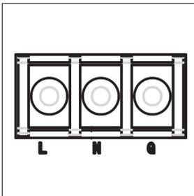
You can plug your AC loads directly into the receptacles on the inverter's AC Side. You can also hardwire (permanently connect) the AC output from the AC hardwire terminal through the AC knockout into a load sub-panel or additional AC outlets powered by the inverter. From left to right, the terminal block indicates: Live/Hot (L), Neutral (N), and Ground (G).
